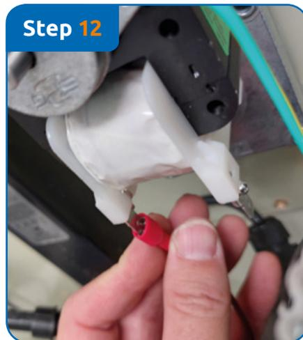
Attach the supplied cable shoes over the contacts on the motor (it does not matter where the brown and blue wire are).
