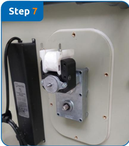
Remove the locknut completely and carefully remove the motor from the shaft. Make sure that the seal ring around the shaft does not fall and you lose it. Now place the new motor over the shaft and screw the motor back to the filter wall with the hex head bolts as it was (Photo step 6)
