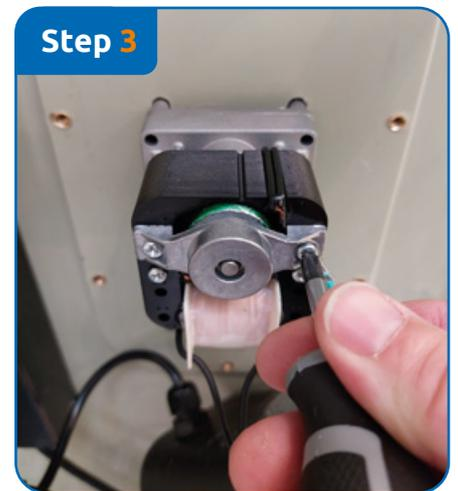
Unscrew the ground wire and put the cover with the wires stuck in it to one side.
