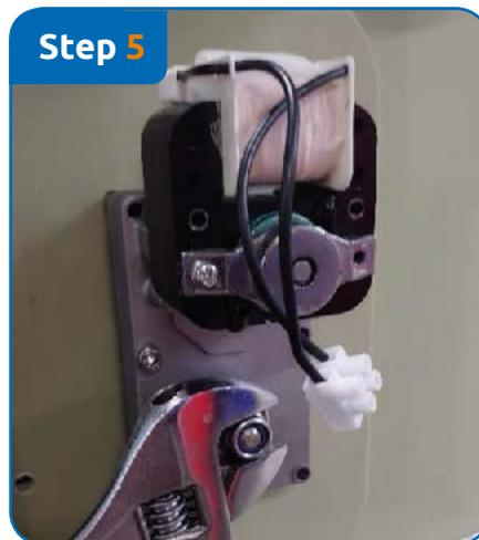
Loosen the locknut (17mm) of the shaft while holding the drum so that it cannot rotate.
