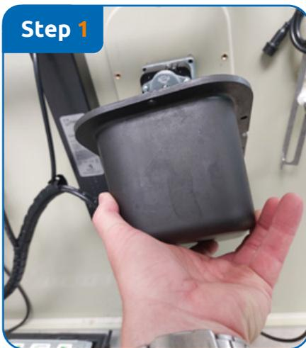
Start with removing the cap of the motor by unscrewing the hex head bolts.
