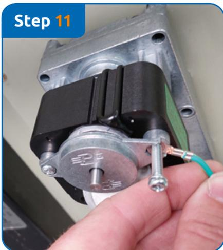
Screw on the motor in this position, reconnecting the ground wire.
