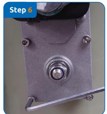
Now loosen the bolts holding the motor to the filter
