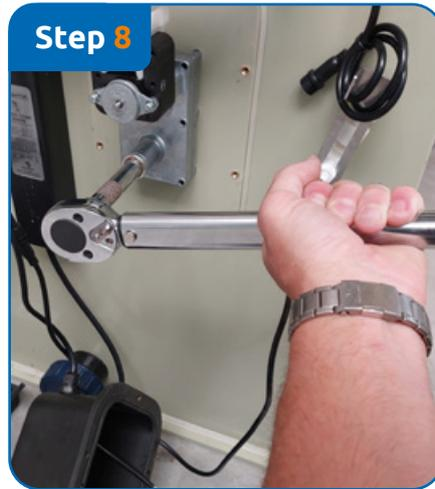
Now tighten the locknut of the shaft with a torque wrench at 65 Nm; again make sure that you (better yet, someone who helps) hold the drum so that it cannot rotate with it.
